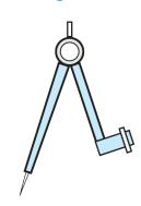
We use a compass to draw a circle. One arm of the compass has a metal point while the other arm has a place to fix a pencil. A pencil of a suitable length is fixed to the compass.
