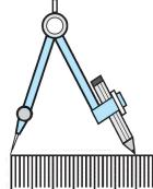
To draw a circle of a given radius, a distance equal to the radius is kept between the pencil point and the metal tip of the compass. In the accompanying diagram, this distance is 3 cm. Therefore, the radius of the circle drawn using this distance is 3 cm.
