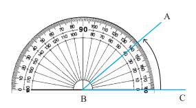
3. The angle is measured starting from the zero on that side of the vertex on which the arm of the angle lies. Here, the arm BC is on the right of the vertex B. Therefore, count the divisions starting from the 0 on the right. See which mark falls on arm BA. Read the number on that mark. This number is the measure of the angle.
