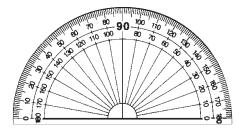
A protractor is used to measure an angle and also to draw an angle according to a given measure.
