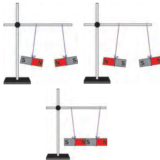
15.11 : Attraction and repulsion in magnets
