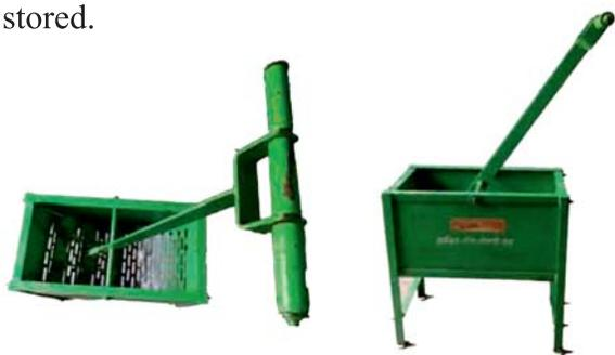
Fig. 1.27 b Groundnut sheller (Hand operated)
