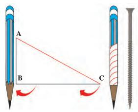
12.4: The screw as an inclined plane
