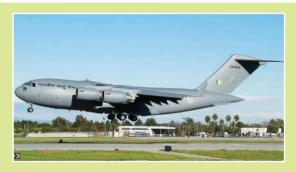
C 17: The aircraft is capable of carrying a payload of 40-70 tons up to a distance of 4200-9000 km in a single hop.
