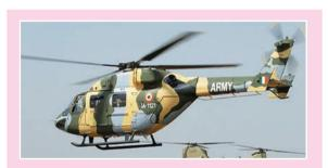
**Dhruv:** This is an Indian origin helicopter for transportation. This helicopter can work in mountainous area effectively up to the height of 6000 m.
