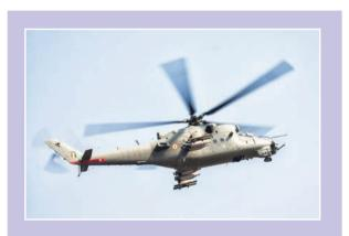
MI 25/MI 35: Twin engine turboshaft, assault and anti armour helicopter.
