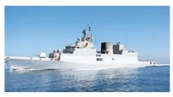
**Corvette:** It is a fast, lightly armed warship which is smaller than a frigate and larger than a coastal patrol craft often armed for antisubmarine operation.
