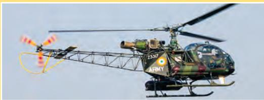
**Cheetah :** Single engine turboshaft, FAC / casevac helicopter of French origin.
