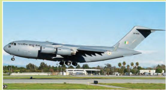
**C 17** : The aircraft is capable of carrying a payload of 40-70 tons up to a distance of 4200-9000 km in a single hop.
