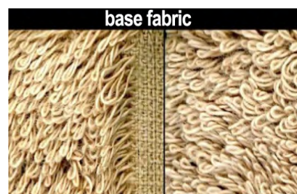
Pic. No. 6.14 Uncut pile weave
