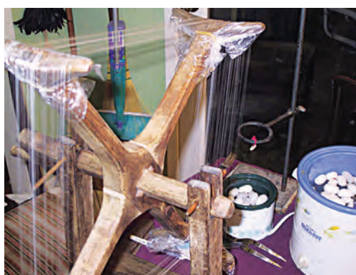
Picture No. 2.9 Filature Operation
