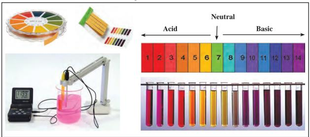
5.4 Measurement of pH: universal indicator and pH meter
