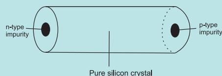
The impurities grow on either side of the crystal after heating in a furnace. Electrons and holes combine at the center and the depletion region develops. A junction is thus formed. Electrodes are inserted after cutting transverse sections and hundreds of diodes are prepared. All semiconductor devices, including ICs, are fabricated by 'growing' junctions at the required locations.
