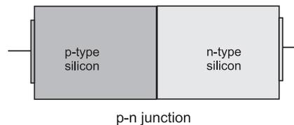
Fig. 14.15: Schematic structure of a p-n junction.
