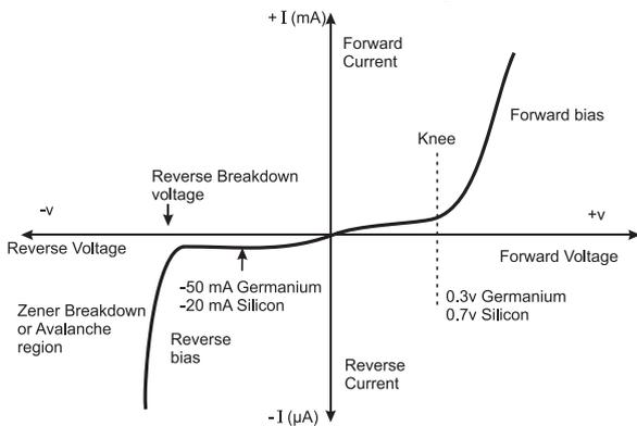
Fig. 14.22: Asymmetrical current flow through a diode.
