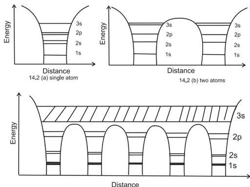
Fig. 14.2: Potential energy diagram, energy levels and bands.
