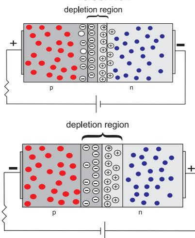
Fig. 14.19: Forward biased and reverse biased junction.
