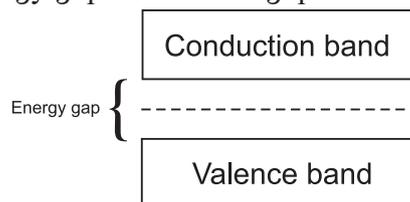
Fig. 14.4: Energy bands for a typical solid.
