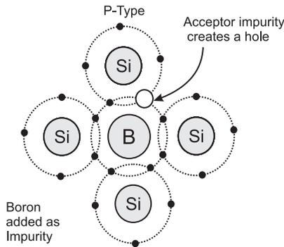
Fig. 14.13: A trivalent impurity in a silicon crystal.
