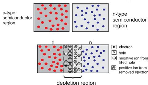
Fig. 14.17: Potential barrier and the depletion layer.
