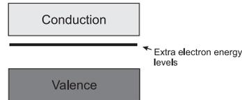
**Fig.14.11: Schematic band structure of an n-type semiconductor.**
