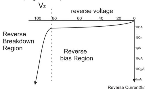
**Fig. 14.26: Reverse biased characteristic of a diode.**
