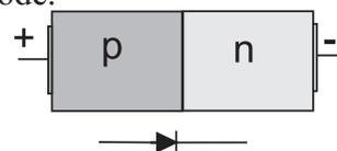
Fig. 14.20: Circuit symbol for a p-n junction diode.
