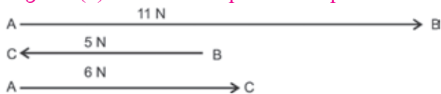
Fig 2.4 (b): Resultant of anti-parallel forces.
