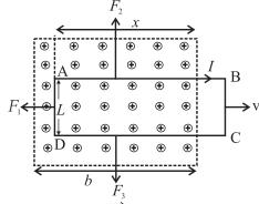
$\oplus$  Magnetic field  $\overrightarrow{B}$  into plane of the paper Fig. 12.9 (a): A loop is moving out of magnetic
