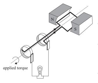
Fig. 12.8 (a): Schematic of a Generator.
