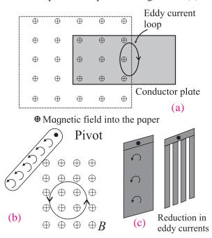
Fig. 12.10: (a) Eddy currents are induced in solid conductor plate, (b) Conducting plate swings like a pendulum, (c) Reduction in eddy currents due to discontinuous structure of a plate. 12.11 Self-Inductance:
