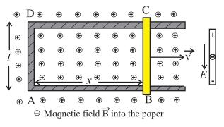
Fig. 12.5: A frame of wire ABCD in magnetic field  $\vec{B}$ . Wire BC is moving with velocity  $\vec{v}$  along x- axis.
