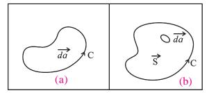
Fig. 12.4: (a) Small element of area  $\overline{da}$  bounded by a curve considered in anticlockwise direction. (Right-handed screw Rule), (b) Finite surface area  $\overline{S}$ .
