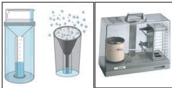
(ii) Self recording rain gauge
