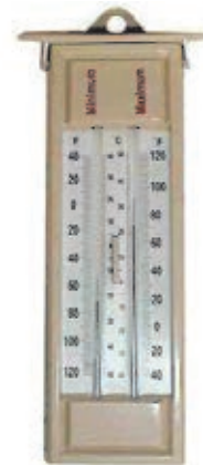
Fig 2.2 : Minimum and maximum thermometer
