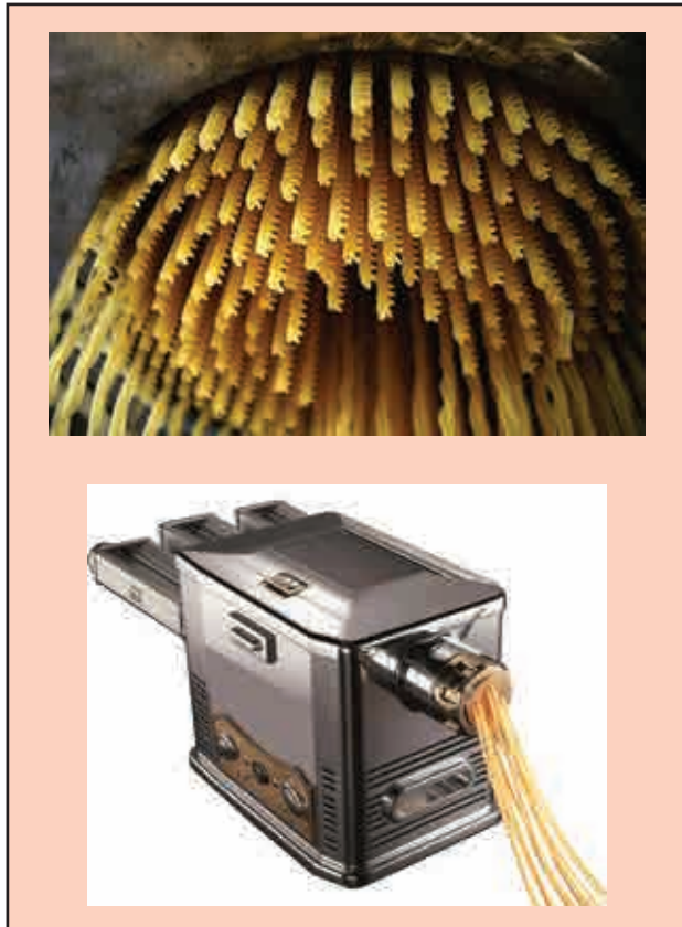
Fig. 10.3a : Pasta making machine (Extrusion of Pasta)
