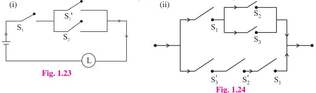
Q.4. Write the symbolic form of the following switching circuits construct its switching table and interpret it.
