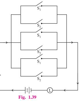
Q.17. Represent the following switching circuit in symbolic form and construct its switching table. Write your conclusion from the switching table.
