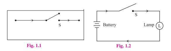
In figure 1.2, we consider a circuit containing an electric lamp L, controlled by a switch S.
