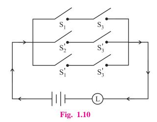
Ex.3. Give an alternative arrangement for the following circuit, so that the new circuit has minimum switches.
