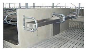
Fig. 2.18: Modern automated water trough
