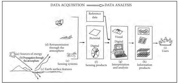
Fig. 8.1 : The process of remote sensing
