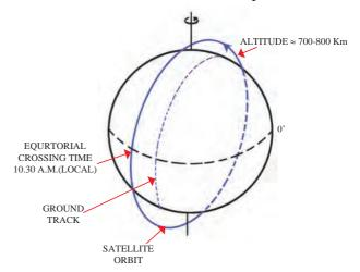
Fig. 8.5 : Orbit of a remote sensing satellite
