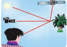
Fig. 8.2 : Passive Remote sensing – Sun is the primary source of illumination. Carried out by remote sensing satellites which record data in the visible and near infra-red wavelengths. e.g. IRS and Cartosat series of satellites launched by ISRO.
