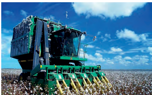
Picture No. : 2.2 Mechanical Picking
