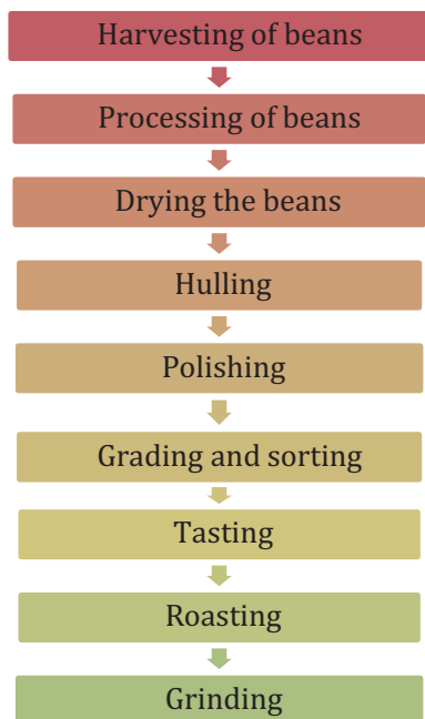
Fig. 12.20 Flow chart of coffee production
