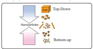
Fig. 16.6 : Schematic illustration of the preparation of nanoparticles
