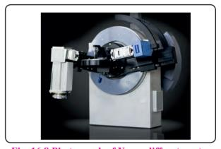
Fig. 16.8 Photograph of X-ray diffractometer
