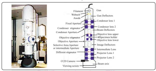
Fig. 16.11Transmission electron microscope (TEM)
