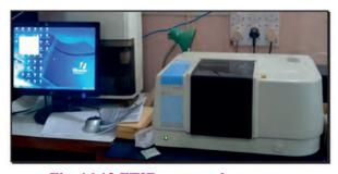
Fig. 16.12 FTIR spectrophotometer
