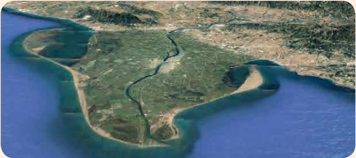
Fig.3.7 B) Cuspate delta : These deltas have a kite like appearance because the material is deposited evenly on either side of the main channel. e.g. Ebro delta, Spain.
