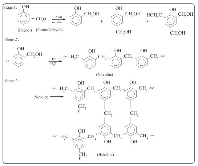
Fig. 15.3 Preparation of Bakelite
