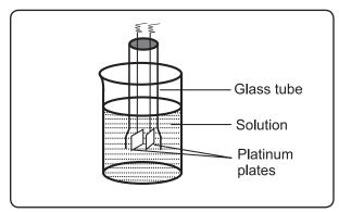
Fig. 5.2: Conductivity cell
