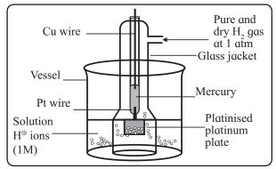
Fig. 5.6: Standard hydrogen electrode
