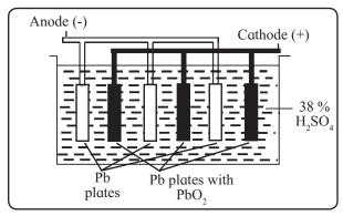
Fig. 5.9: Lead storage cell
