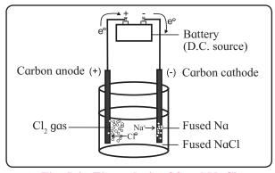
Fig. 5.4: Electrolysis of fused NaCl
