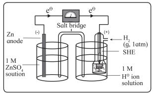
Fig. 5.7: Determination of standard potential using SHE
