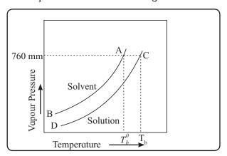
Fig. 2.6 : Vapour pressure-temperature of pure solvent and solution
