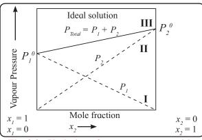
Fig. 2.2 : Variation of vapour pressure with mole fraction of solute
