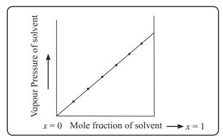
Fig. 2.5: Variation of vapour pressure of solution with mole fraction of solvent
